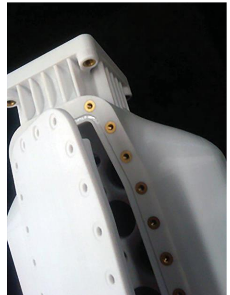
Figure 1: Brass threaded inserts installed in an FDM part.
