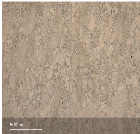
Microstructure solution annealed Etched with etchant Kallings 2
