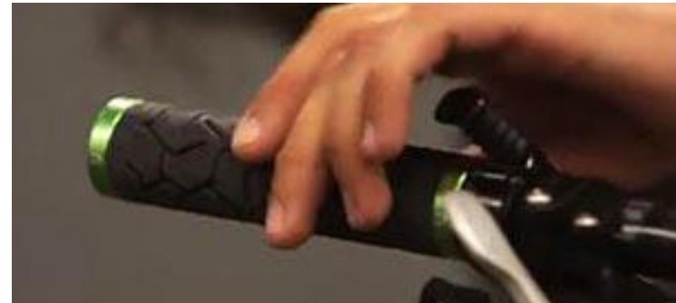
Functional handlebar grip prototype produced using rubber-like TangoBlackPlus.
