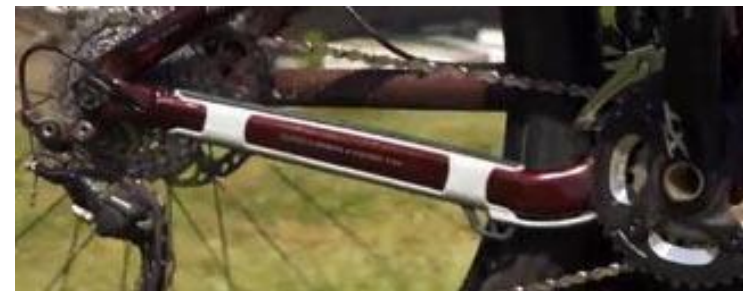
Chain protector and sound guard produced using Digital ABS and rubber-like TangoBlackPlus.
