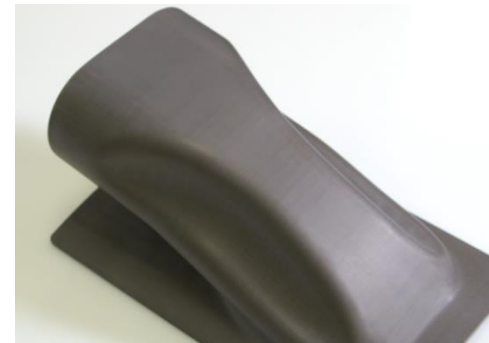
Typical Epoxy-Sealed Surface
