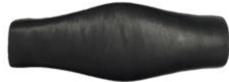
Filament-wound duct (Top = Sacrificial Tool, Bottom = Carbon fiber wound over tool)
