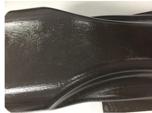
Typical Quickskin-Sealed Surface
