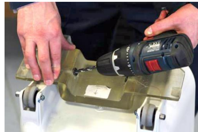
Drill guide made from FC720 material.
