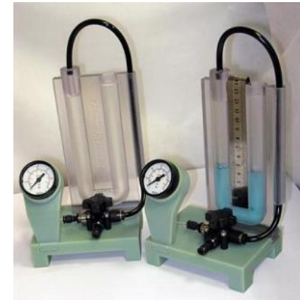
Pressure gage using Digital ABS™ and VeroClear™.
