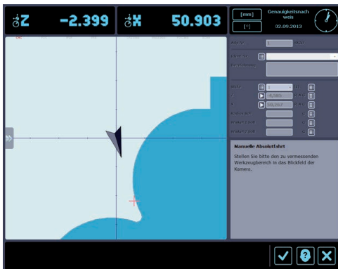
Navigation system »compass« for a quick and comfortable axis adjustment and positioning of the nominal value
