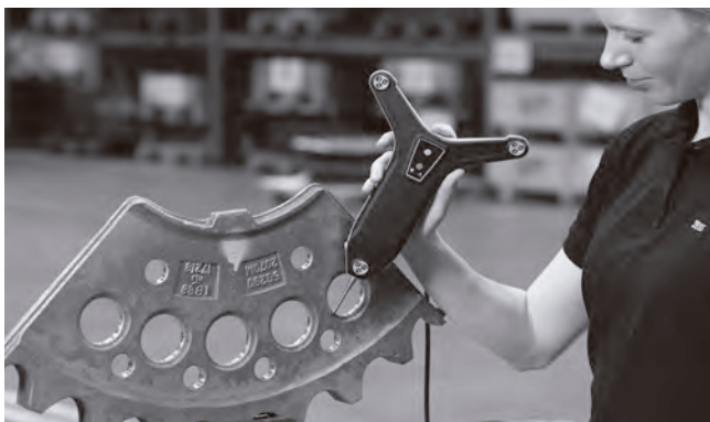
Hand-held touch probe ZEISS T-POINT - the ideal portable coordinate measurement machine for easy single point measurements
