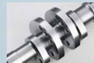
Camshaft after finishing
