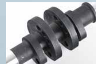
Camshaft before finishing
