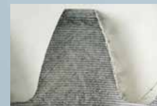
Tooth flank before finishing
