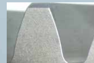
Tooth flank after finishing
