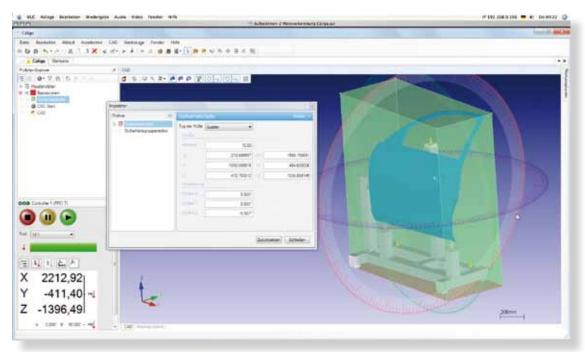
CALIGO automatically generates a safety sheath that can be modified as needed.
