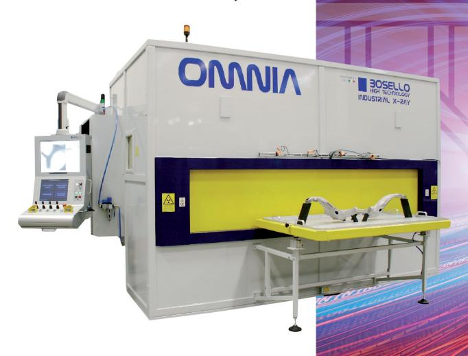
BOSELLO HIGH TECHNOLOGY is pleased to present the latest and innovative solution for Radioscopic inspection of medium/big size castings.
