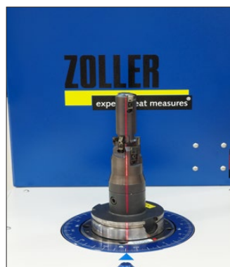
Laser marking for quick help and exact reading of values
